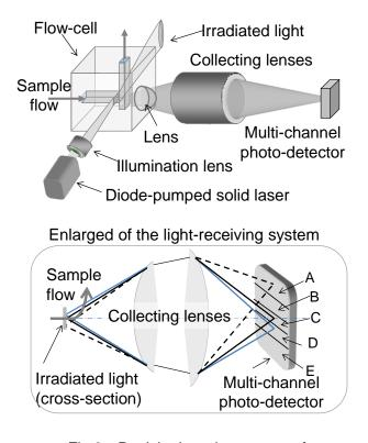
Fig.3 Particle detection system of liquid-borne
