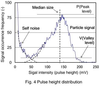
for test particle-sensing signals.
