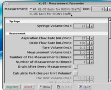
One aspiration action can be used for multiple measurements (within 25 mL)
