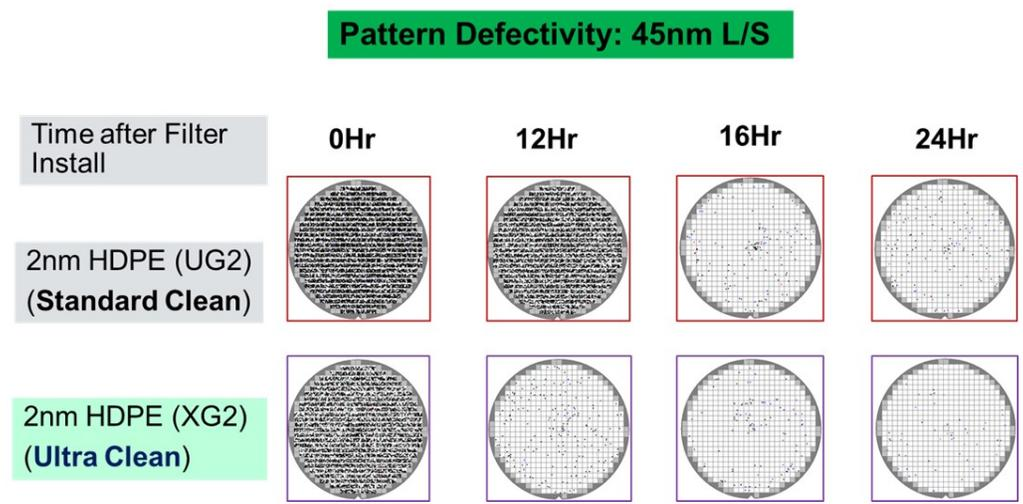
Figure 6. Specific pattern defectivity observed for wafers processed at different duration of use of the XG2 Ultra Clean and UG2 Standard Clean filters in PR filtration.
