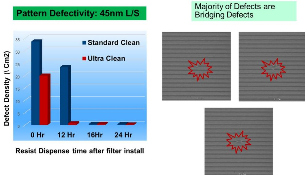
Figure 7. Relative defect density for patterned wafers processed during use of XG2 Ultra Clean filter vs. UG2 Standard Clean filter, with images of bridging defects observed
