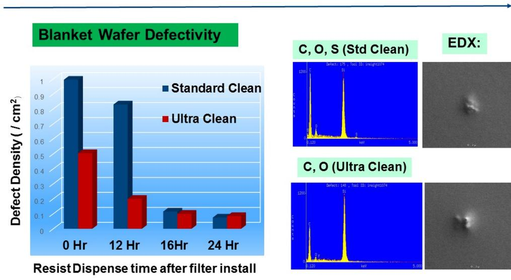
Figure 5. Relative defect density for blanket wafers processed during use of XG2 Ultra Clean filter vs. UG2 Standard Clean filter, with EDX data for defects detected in each case.
