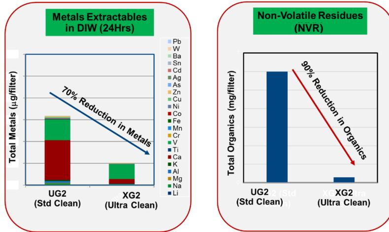
Figure 3. Relative metal and organic extractables levels obtained for UG2 and XG2 filters.
