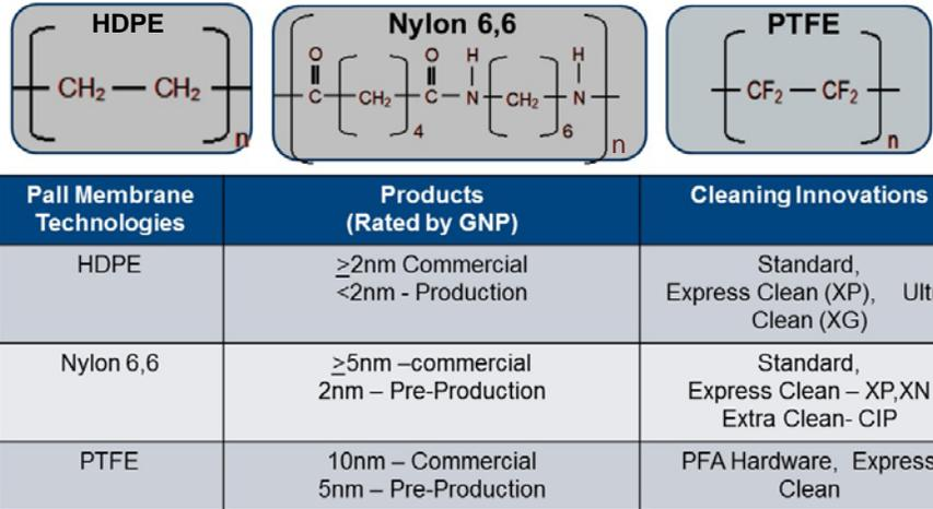
Figure 1. Finer membranes available from Pall Corporation for lithography applications (Note: “GNP” refers to gold nanoparticles)
