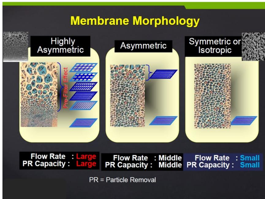
Figure 2. Different types of membrane morphology that may apply for filtration media used in lithography applications.
