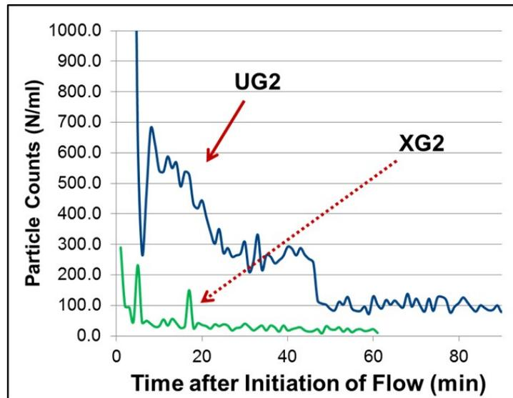
Figure 4. Particle rinse-in curves for particles 30 nm and larger, for capsules subjected to 300 mL/min flow of 70/30 PGME/PGMEA solvent in recirculation.
