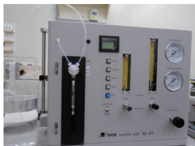
Fig. 1. (Color online) Automatic sampling module RION XL-21.
