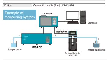
For operation control of particle sensor and display of measurement data
